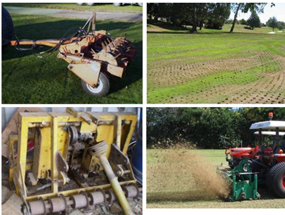
Fig. 2. Photos of mechanical tools used in the golf industry to mitigate SWR. Tumble corer (top left) for aeration and decompaction for soils of golf course fairways (top right). Vibramole (bottom left) and de-thatcher or scarifier (bottom right). Photos by Geoff Walker.
