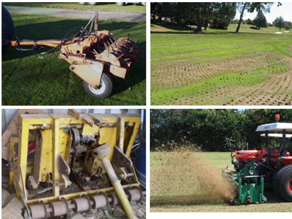
Fig. 2. Photos of mechanical tools used in the golf industry to mitigate SWR. Tumble corer (top left) for aeration and decompaction for soils of golf course fairways (top right). Vibramole (bottom left) and de-thatcher or scarifier (bottom right).
